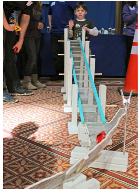
AMT's exhibit: the cars that went down the flat, curved roadway flew off the track, while cars that went down the super-elevated bank followed the track and did not fall off the roadway.
