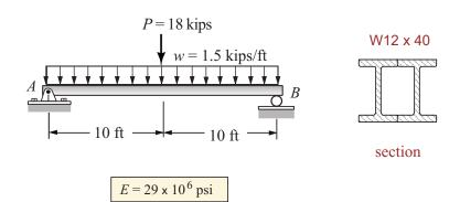
A composite beam is made of two W  $12 \times 40$  welded together. The beam weight is included in the uniform load. Using the given beam dimensions and loads answer the following questions:
