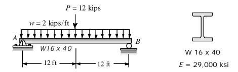
For the simple beam shown the beam weight is included in the uniform load. Determine the maximum deflection and the slope at A (in radians).
