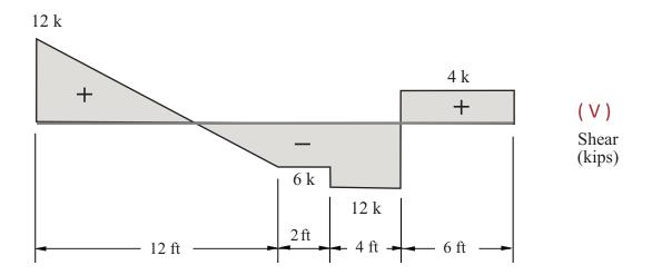
The shear force diagram of a determinate beam is given as shown. Knowing that all lines in the diagram are straight and there are no concentrated moments (couples) anywhere in the beam, the maximum magnitude of the bending moment (ft-kips) in the beam is most nearly:
