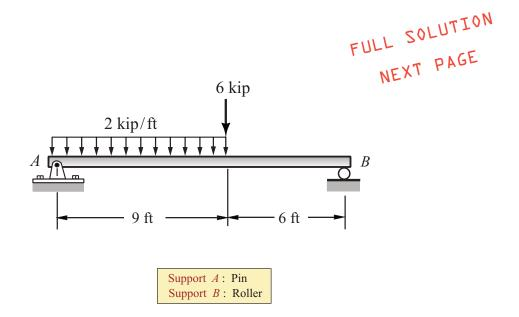
A simply supported beam is loaded as shown. Using the given support conditions, the maximum bending moment (k-ft) in the beam is most nearly:
