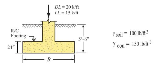
Allowable soil pressure:  $\sigma_a = 3,750 \text{ lb/ft}^2$
